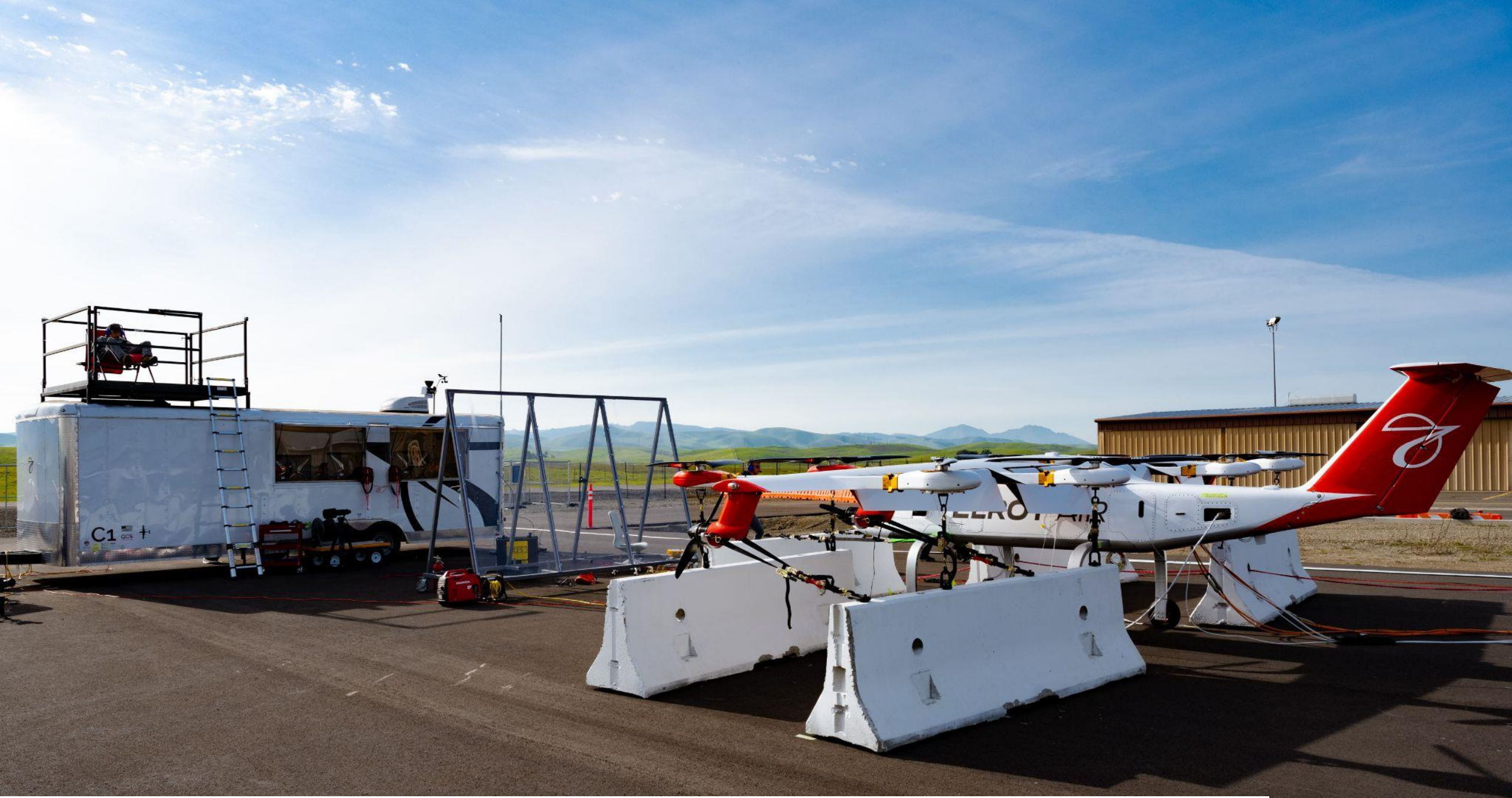
Chaparral in tie-down testing (Byron Airport, CA)
